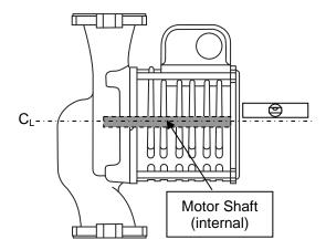
Warning! "Mount with motor shaft horizontal and terminal box above centerline ( $C_L$ ) only!"
